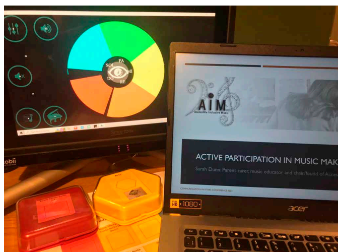
Photo shows an eye gaze device on the left of the image with an eye gaze musical instrument on the screen (eye harp). There is a multicoloured circle on the eye gaze device screen and different symbols signifying volume, a grand piano image to signify instrument choice and an equaliser symbol. There is a red and yellow switch button underneath the eye gaze device and a laptop screen to the right with the title page of the workshop on the screen 'Active Participation in Music Making Using AAC'.
