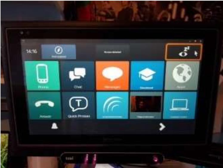
The electronic communication aid acts as a voice for M. He has a Grid Pad with Grid 3 software and uses the Fast Talker grids. He accesses it by EyeGaze using the in-built camera.
