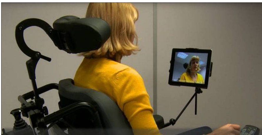
Mounting a communication aid on a power wheelchair (photo supplied by MND Association 2014)
