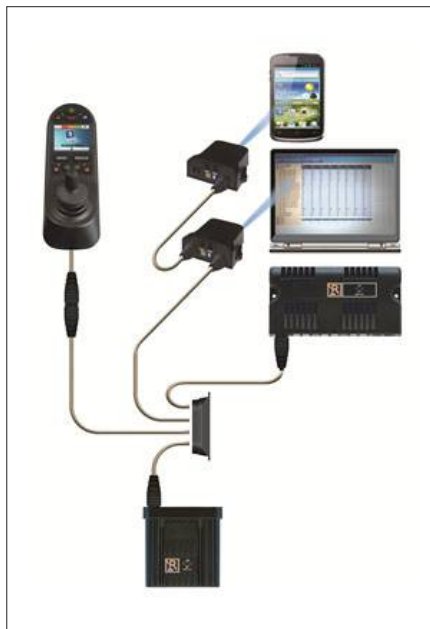
Bluetooth pairing with and R-net joystick control and Android device (Penny & Giles Controls Ltd 2013)
