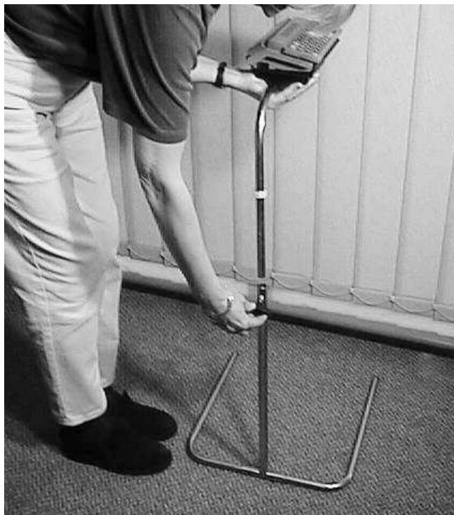
Lightwriter and 'L' pole are then fitted into floor stand
