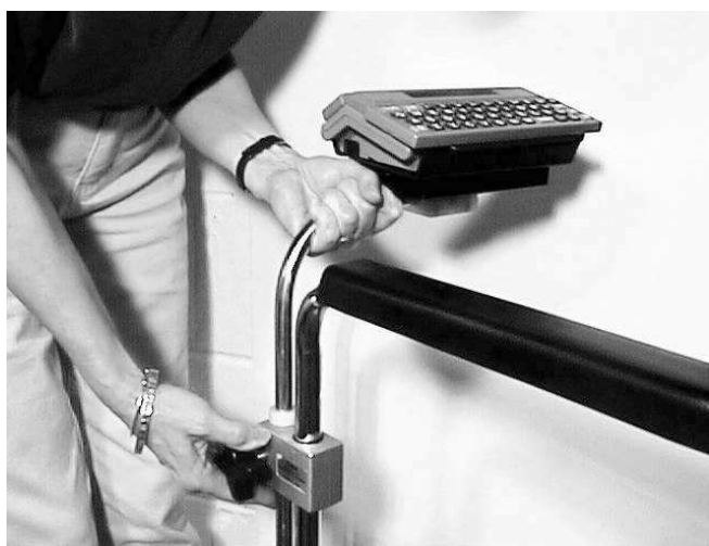
Lightwriter and 'L' pole are removed from wheelchair mount
